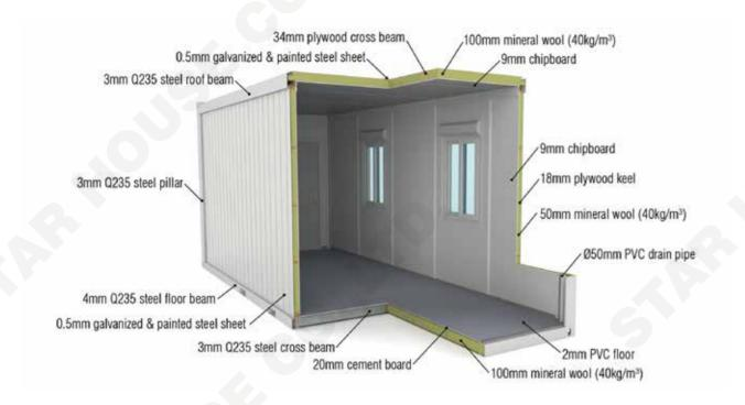
Flat pack container is a multi-function standard container, which dimensions conform to the ISO container transportation. It is a prefabricated building structure composed of roof, floor and pillars. This structure enables the containers to combine in longitudinal and transverse directions without limits, or be stacked in 2 floors or 3 floors in height.
